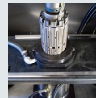
INTEGRATED AIR SIZING SYSTEMS CONTROL THE ACCURACY OF BOTH ROUGHING AND FINISHING PROCESSES.
